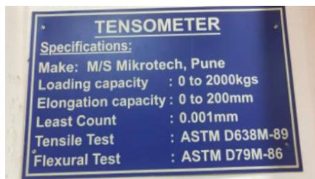
**Figure 4.4 Tensometer experimental setup Specifications**
