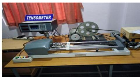
**Figure 4.5 Electronic tensometer for tensile & flexural testing**
